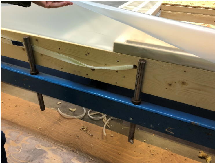
Figure 16 Lifting loops like this might possibly be left in the mounted structure, but this would have to be studied.
