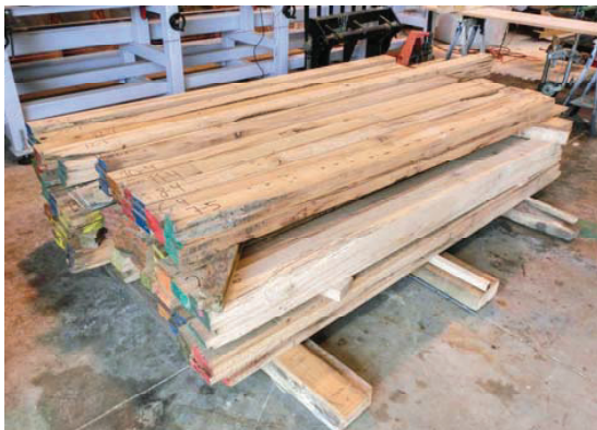
Figure 2: Recovered sawn timber boards
