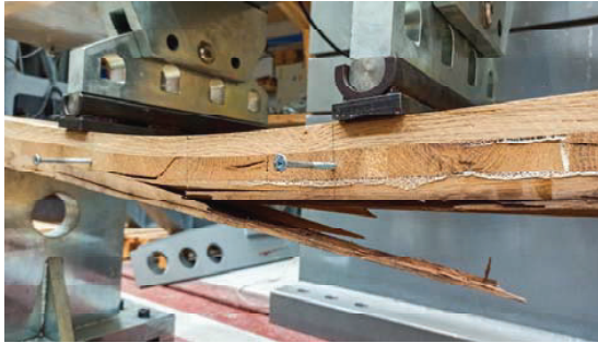
Figure 6: CLT panel failure in tension
