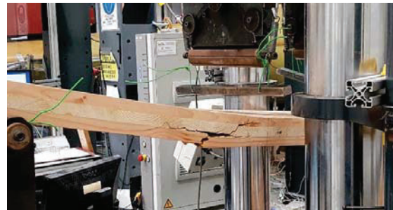
Figure 6: Bending failure of hybrid CLT panel
